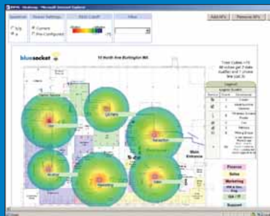
BlueView enables you to determine the location of rogue access points, users and attackers and graphically represents RF coverage.
