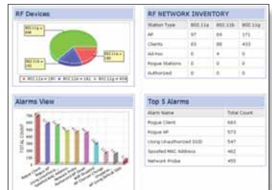
View real-time updates of security and operational status, and performance exceptions. Determine how your WLAN (spectrum, channels) is being used, where security holes are, and when intruders are trying to access your WLAN.
